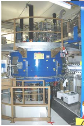
a) COMET, the new dedicated medical proton accelerator
