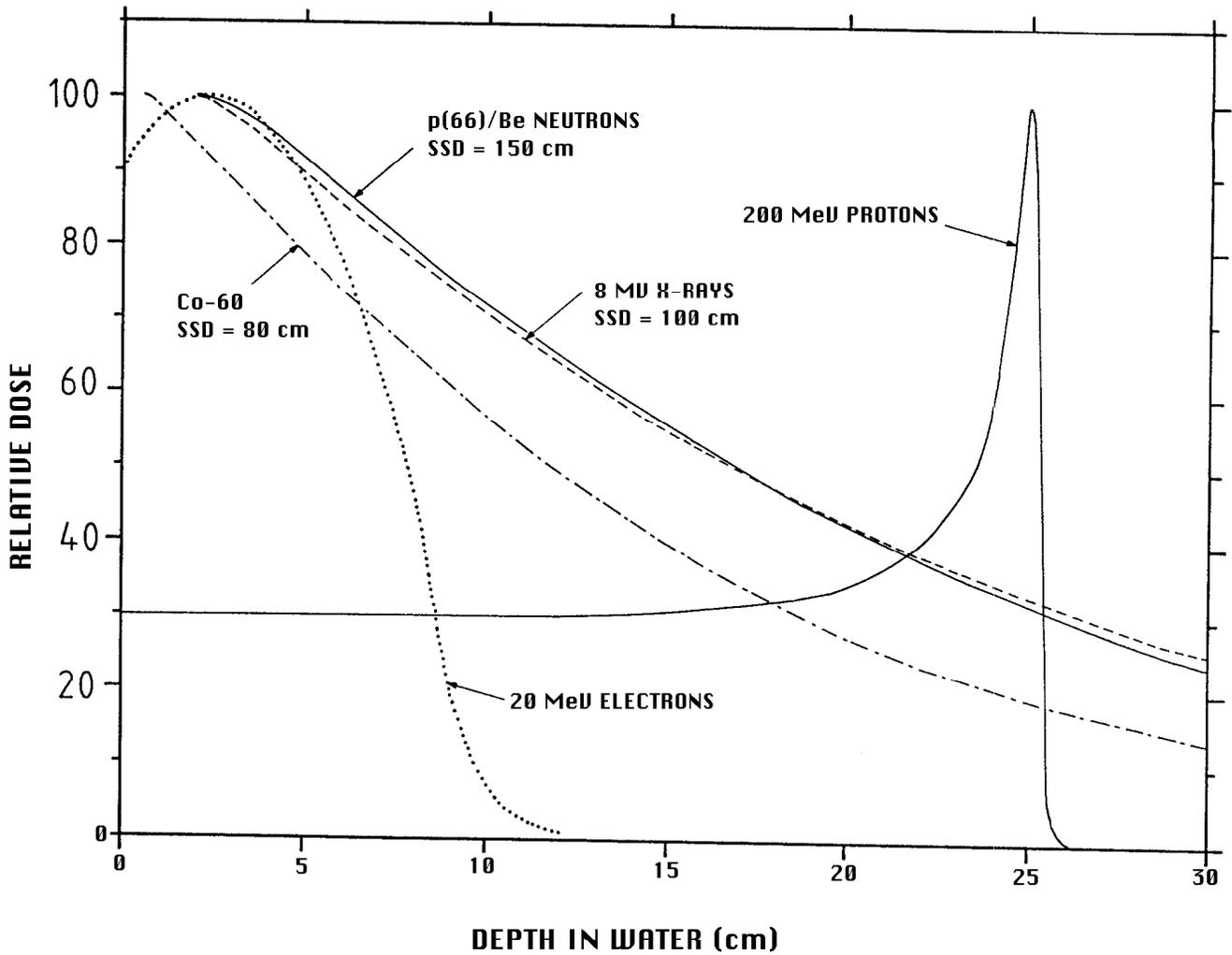
The depth dose distribution was measured in an uncollimated beam in a water phantom with a 0.3 cm<sup>3</sup> TE ionization chamber. Also shown is the depth dose curve for their isocentric p (66/MeV) / Be (40 MeV) neutron therapy beam.
